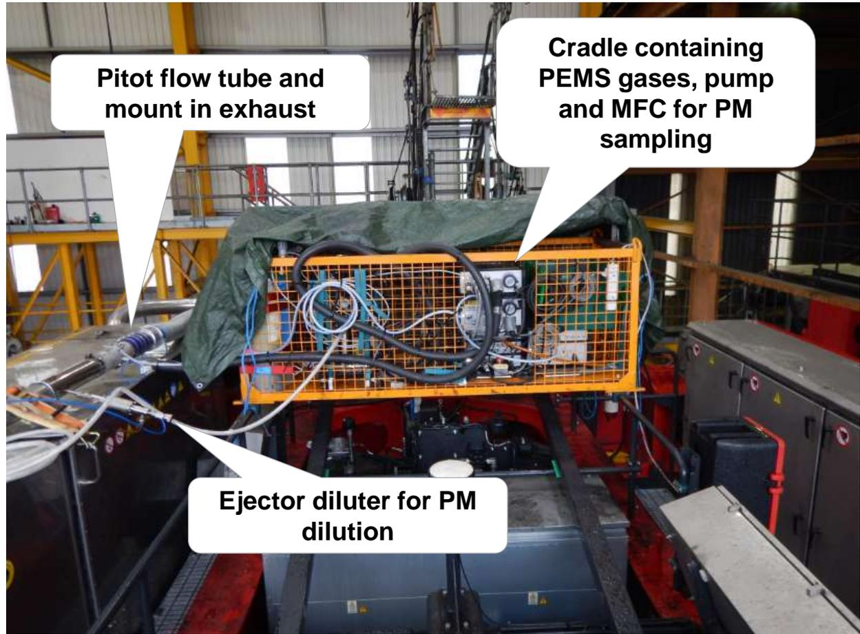
**Pitot flow tube and mount in exhaust**
