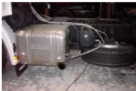
Exhaust Pitot flow meter, installed at the exit of the tailpipe
