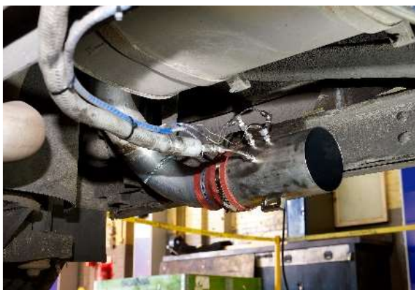
Exhaust Pitot Flow Meter, installed at the exit of the tailpipe
