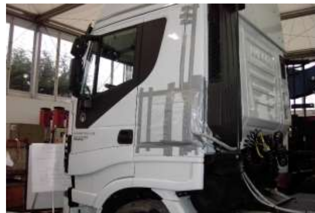
Heated sample transfer line direct from exhaust to PEMS via left side hatch
