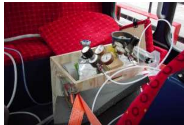
Service gases, crated and anchored between seats
