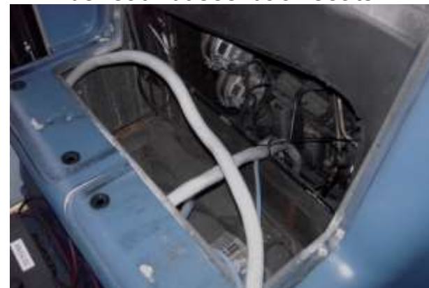
Sample Heated Transfer Line direct from exhaust to PEMS via void beneath buses' back seats
